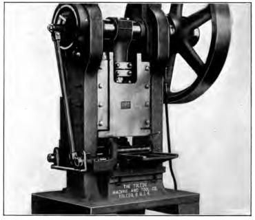
Fig. 4. Double-roll Feeding Mechanism applied to Straight-sided Press
